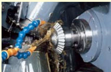
Gear cutting of Straight Bevel Gears
