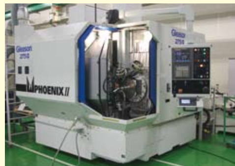
Bevel Gear Grinding Machine (Gleason PH-275HG)
