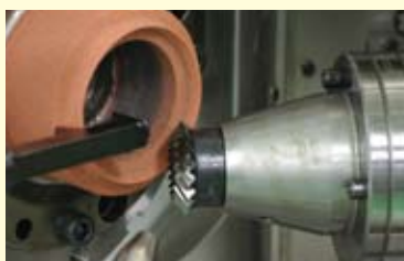
Gear cutting of Spiral Bevel Gears
