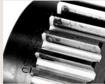
Poor tooth contact and pitting
