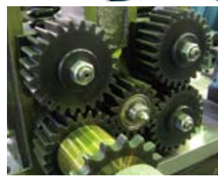
Takashima High-Speed Wire Straightening & Cutting Machines by Takashima Sangyo Co., Ltd. SS Spur Gears are used at the feeder.
