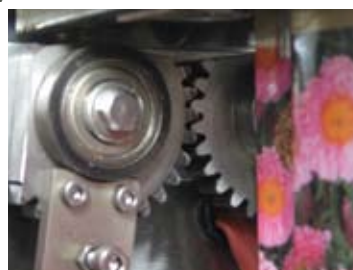
Automatic Packing Machine by New Max SS Spur Gears, segment shaped by secondary operation, are used at the crimping device.
