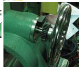
Electric Wire Winder by Sakuma Tekko KK. SS Spur Gears are used at the stopper of handgrip.
